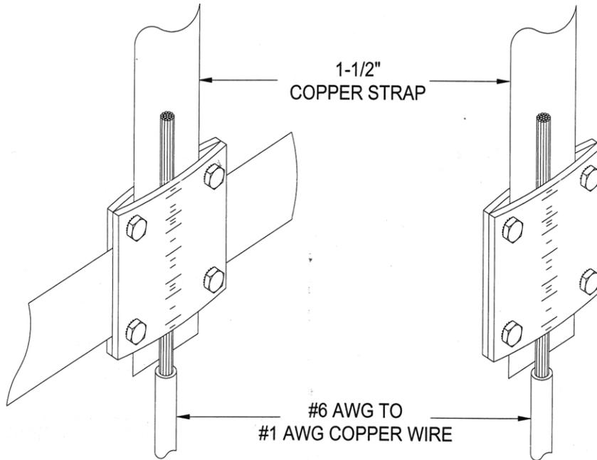
**Figure 20: PPC-1C-112S Transition from copper wire to copper strap.**
