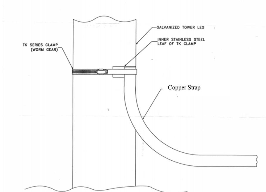
**Figure 3: TK Series Clamp Transition from Tower Leg to Copper Strap**
