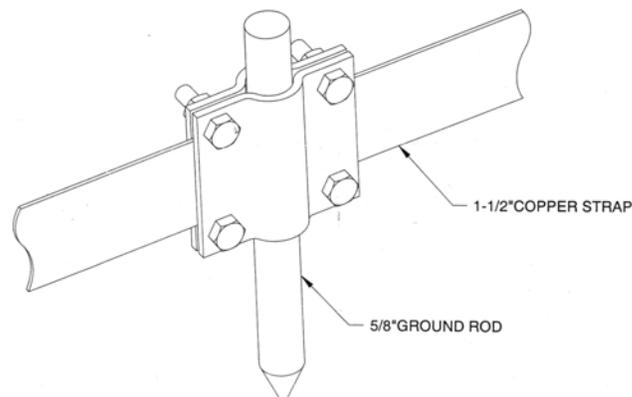
**Figure 19: A PPC-58R-112S Ground Rod to Copper Strap Bonding Clamp**
