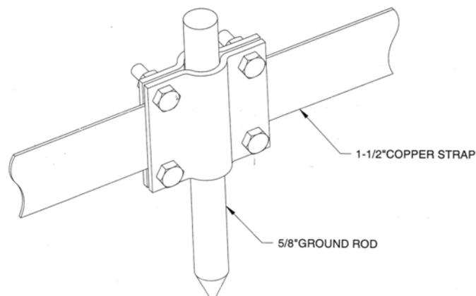
**Figure 2: PPC-58R-112S Ground Rod to Strap clamp**
