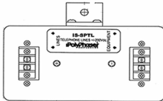
**Figure 24: PPC-IS-SPTL Telephone Protector**
