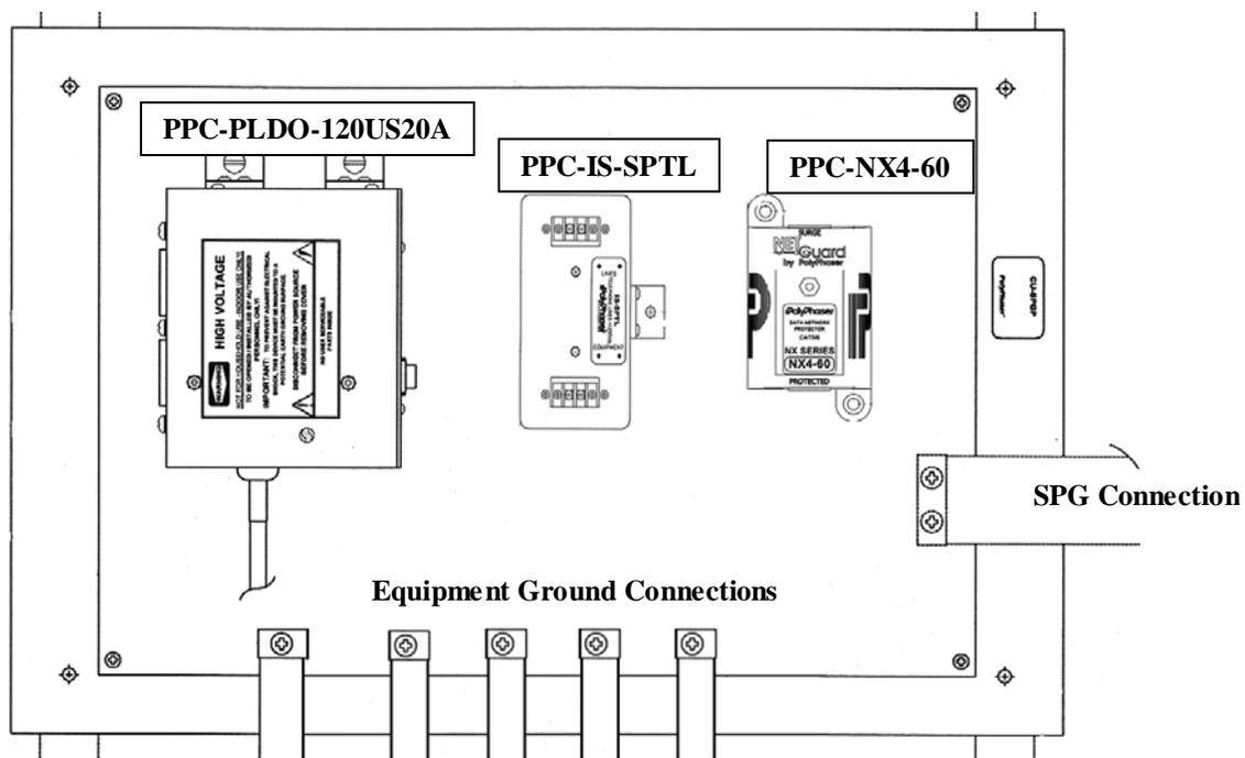
**Figure 22: Single Point Ground Plate with Optional Protectors Mounted**
