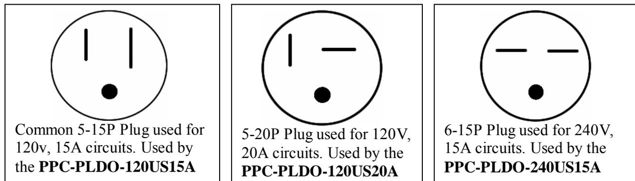
**Figure 23: Plugs Used on the Noted PLDO Protectors**
