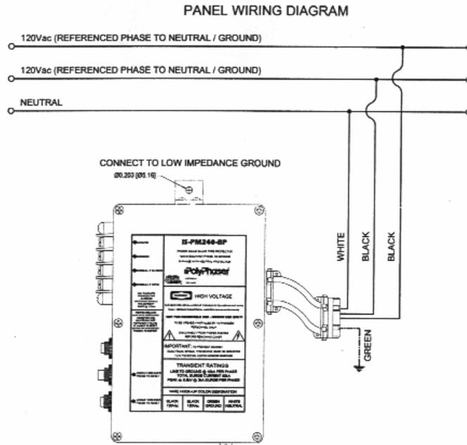
**Figure 17: PM240-BP Whole House Protector Wiring Example**
