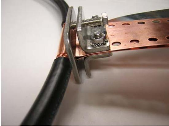
**Figure 9: Completed grounding assembly**
