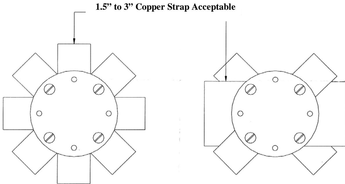
**Figure 4: MSC-3 Copper Strap Bonding Clamp**
